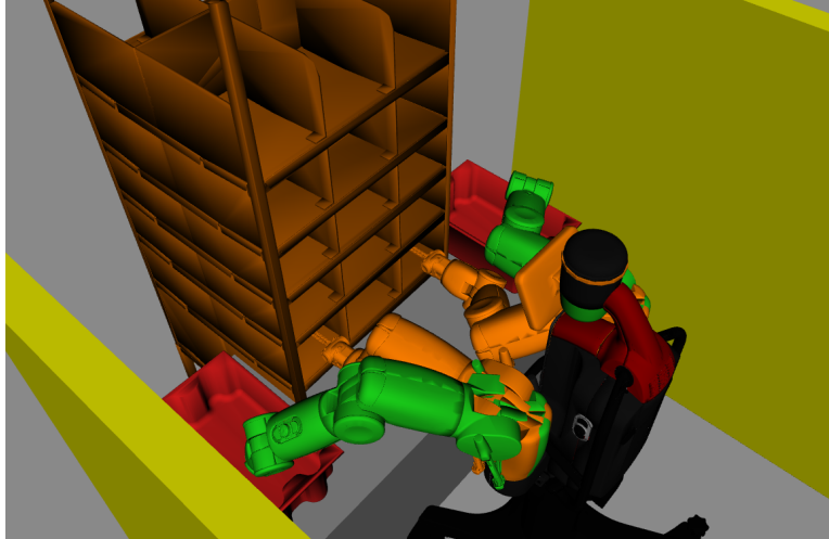
Figure 6.4: Experimental setup of dual-arm shelf picking where the green robot is the start state and the orange robot is one of the goal states. Three walls define the workcell of the robot, and a table and warehouse shelf are in front of the robot.
